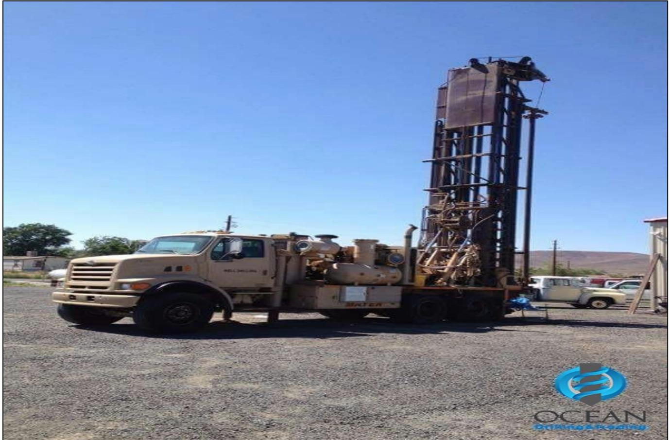
Puits de forage DrillTech 40
