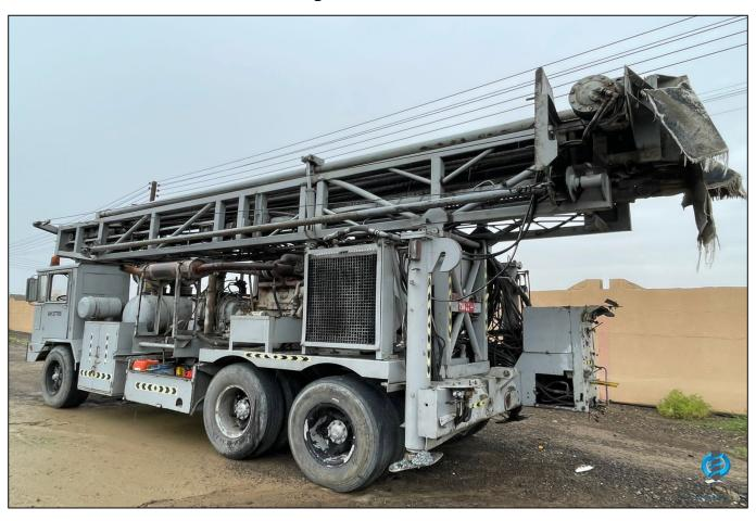
machine in working condition it has 300m drill rod and two hammer and two bits the , the compressor 900/300 and its good
