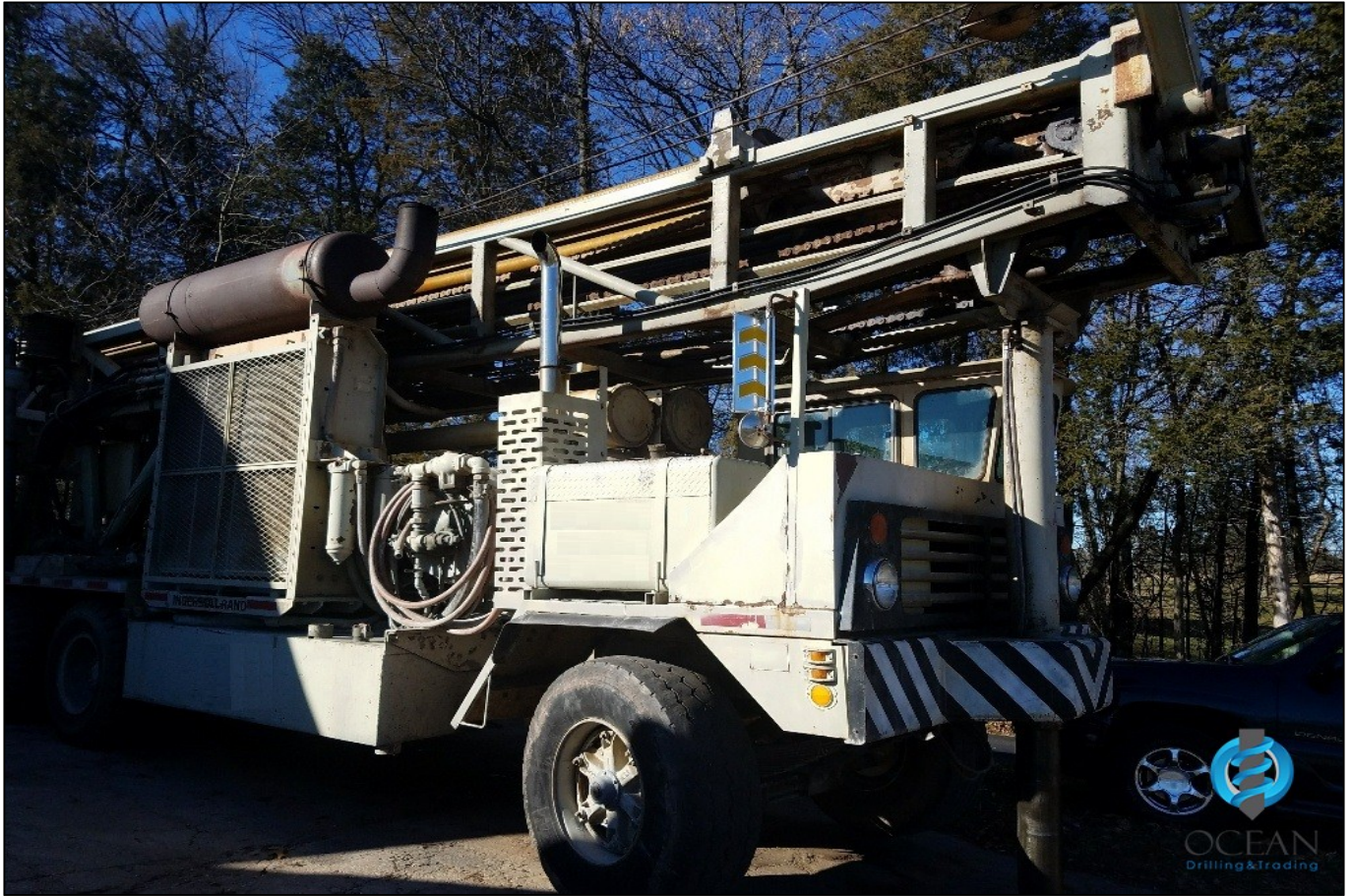
T4W drilling rig Model 84 The Detroit GM12 Compression 350.900
