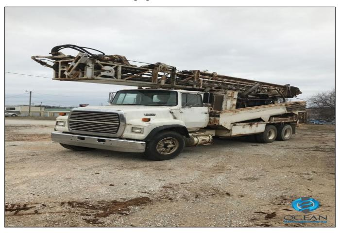
Drilling Rig DrilTech D25
