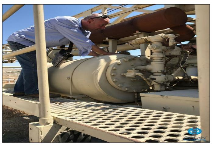
Modern T4-Drilling Rig Ingersoll Rand dm 25 Model 29 Air compressor 759/250 Machine engine cummins is in excellent condition 855 six cylinders 400 hp Number 5 Hammer Drill pipes Atlas 6.5 inches Pipe length 25 feet.
