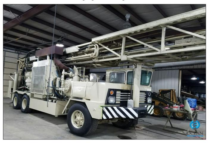
Drilling Rig T4 Long Tower Model 83 Pullback Capacity 38 tons Machine 12 cylinder, Caterpillar power 750 Compressor 350.1050 Power head 2 retary
