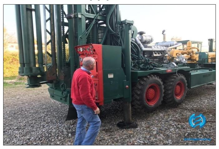
Drilling rig Ingersoll Rand T4W Model 80 again. Machine engine German Deutz 10 cylinder Pump 4 by 5 With 250 meters of drilling pipes.
