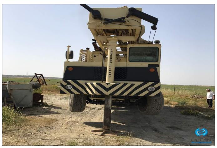
Drilling rig T4W Model 94 Cummins engine Machine 650 Compressor 350.1050 With 300 meters of drilling pipes.
