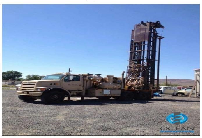
Drilling Wells DrillTech 40 Model 99 Machine engine Caterpillar C-15 Compressor 350.1050 With 120 meters of drilling pipes.
