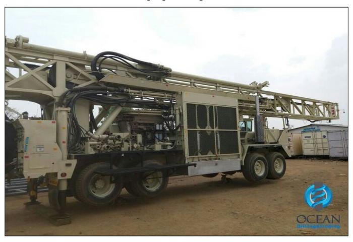
Drilling Rig RD20 Ingersoll Brand Model 2002 Cummins 750 Machine Model 2006 Compressor 1250/350 Very good clean and excellent Maintenance was carried out in 2016 450 meters of drilling pipes.
