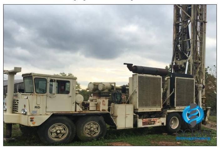
Drilling Rig RD20 American Ingersoll Band Model 97 Machine Engine 3412 Caterpillar Compressor 350, 1050 500 meters of drilling pipes. Truck Engine Caterpillar 3208
