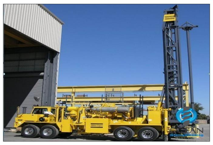
New Drilling Rig Model 2017 Cummins engine 650 Compressor 1070,350. Engine truck cummins410 Power draw 35 tons
