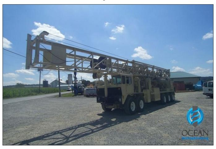
Rig Atlas Atlas Copco American RD20 Model Engine cummins 750 Mechanic Model Compressor 1250 Work hours 9000 The Rig was clean and excellent Maintenance was completed in 2016 With 400 meters drill pipes
