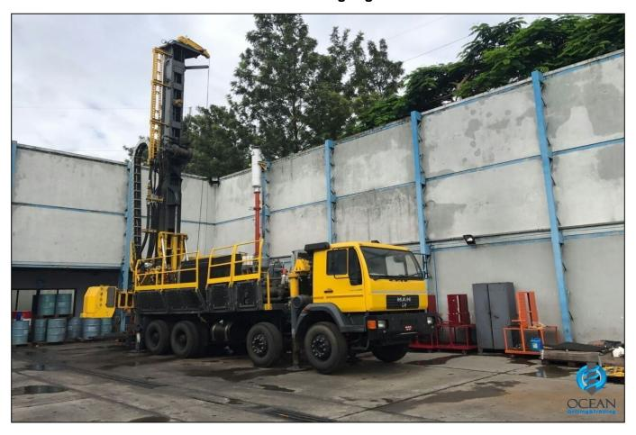
New drilling rig Atlas Copco Drills Model 2017 Compressor 1050 PumpGardendner 4 \* 5
