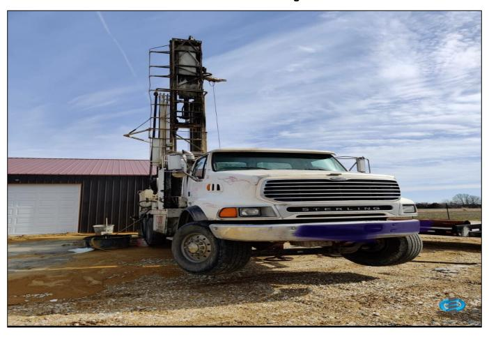
2006 Driltech T25K Sterling Truck 15,000 overall hours 540 HP Cat C-15 Engine rebuilt 1.000/350 Sullair
