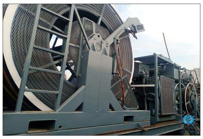
Injector is having 100000 lbs pulling capacity Very highly powered
