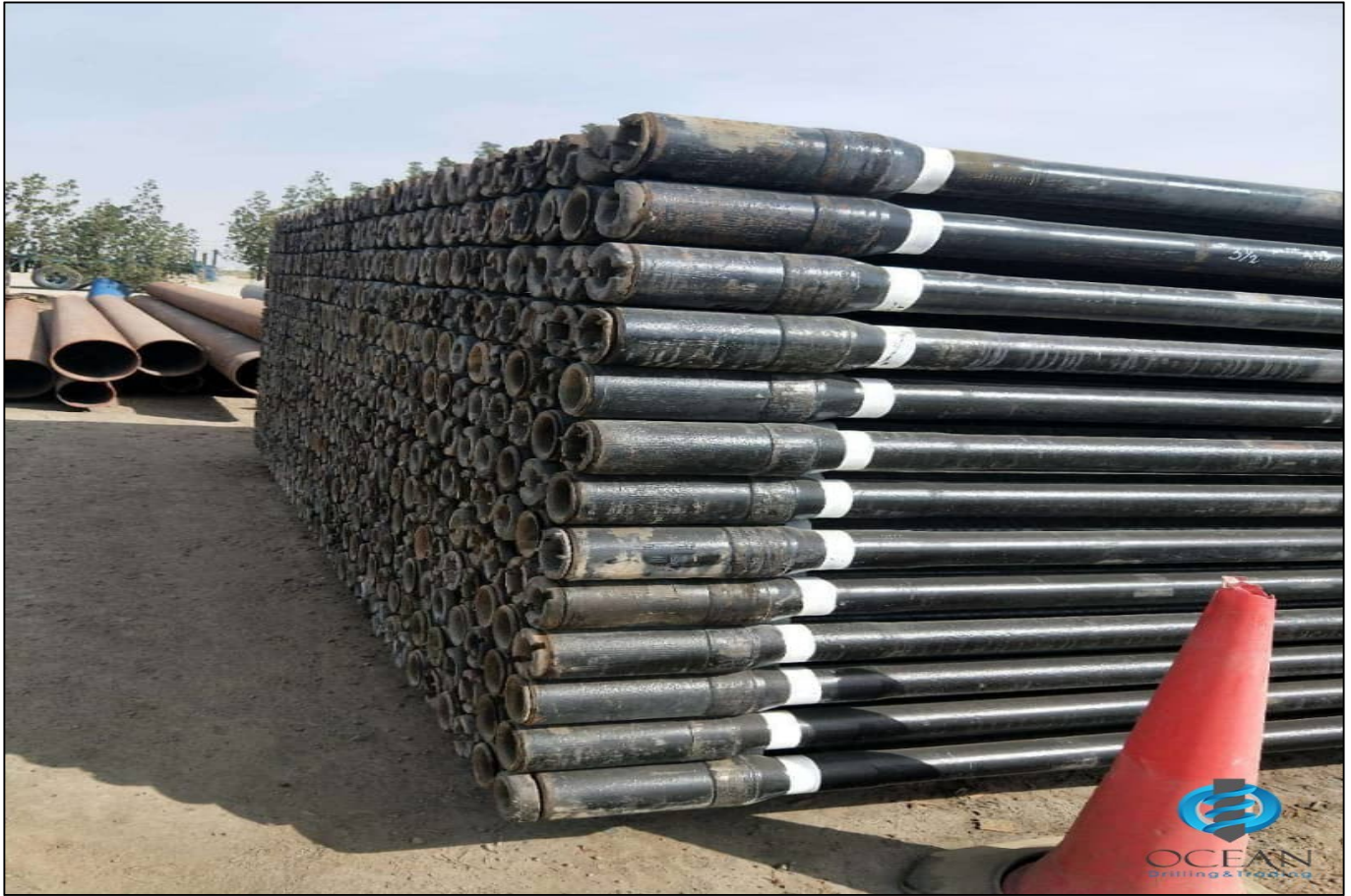
Drill Pipe new american 3 1/2
