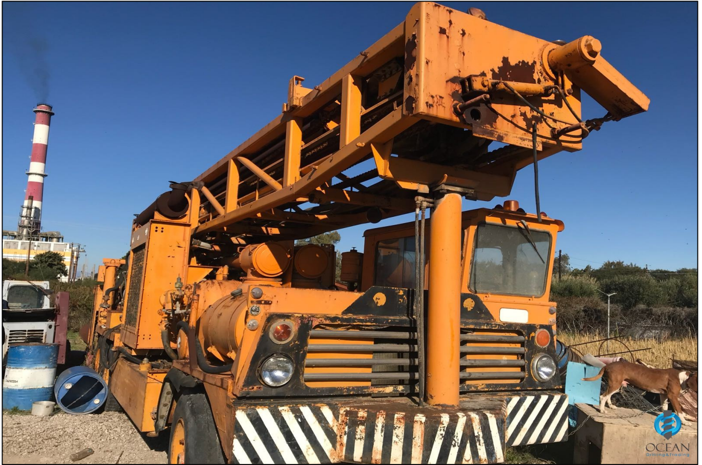
T4W drilling rig Model 82 The Detroit GM12 Compression 300.900
