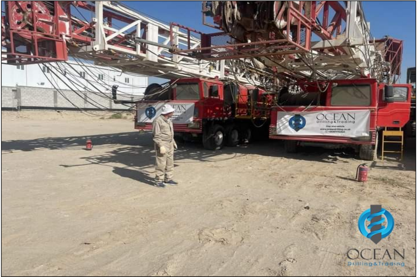
drilling rig 750hp
