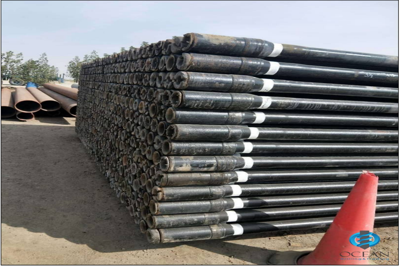
Drill Pipe new american 3 1/2
